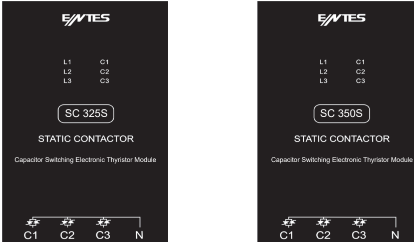
Figure 4: Static Contactor Front View
